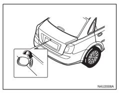
To open the trunk from the outside, insert the key and turn it clockwise in the trunk lock cylinder or use the remote keyless entry transmitter if your vehicle has one.
